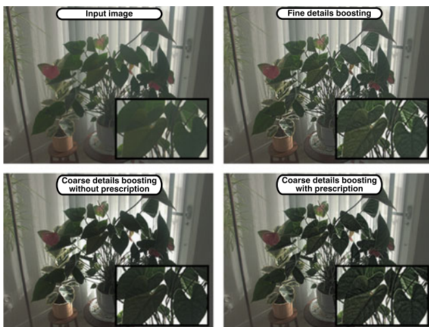
Fig. 8 Contrast editing session in WLS decomposition framework ( \alpha = 1.2 ). Contrast prescription prevents the loss of details in unmodified sub-bands, as a result, previously modified fine details are preserved
